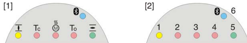
Figure 57: Arrangement and signification of indication lights
