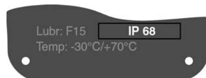
Figure 20: Example: Name plate for enclosure protection IP68
